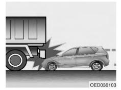
At the moment of an accident, drivers brake heavily with reflex. In such heavy braking, the front portion of the vehicle is lowered by the force of the braking and the vehicle can go under a vehicle with a higher ground clearance. Air bags may not inflate in this situation because impacts may not be delivered or may be delivered with less intensity.
