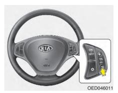
3. Push the SET (-) switch, and release it at the speed you want. The "SET" indicator light in the instrument cluster will illuminate. Release the accelerator at the same time. The desired speed will automatically be maintained.
