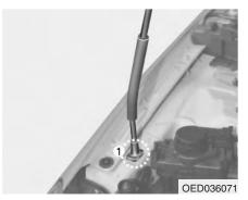
3. Lift the hood and hold it open with the support rod by inserting the free end of the rod into the slot (1).
