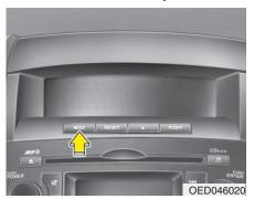
Trip computer is a microcomputercontrolled driver information gauge that displays information related to driving, such as estimated distance to empty, average speed and driving time on the LCD.
