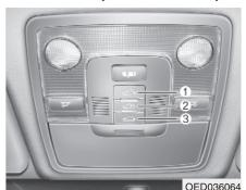
If your vehicle is equipped with a sunroof, you can slide or tilt your sunroof with the sunroof control buttons located on the overhead console.
