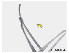
3. Raise the wiper arm and turn the wiper blade assembly to expose the plastic locking clip.
