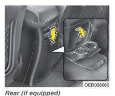
To use the cup holders in rear seat, push the button. Push the cover to close after use.
