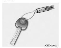
The key code number is stamped on the plate attached to the key set. Should you lose your keys, this number will enable an authorized Kia Dealer to duplicate the keys easily. Remove the plate and store it in a safe place. Also, record the code number and keep it in a safe and handy place, but not in the vehicle.
