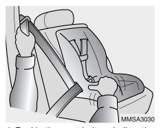
4. Buckle the seat belt and allow the seat belt to take up any slack. After installation of the child restraint system, try to move it in all directions to be sure the child restraint system is securely installed.
