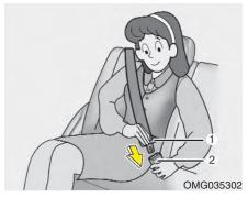
3. Insert the tongue plate (1) into the open end of the buckle (2) until an audible "click" is heard, indicating the belt is locked in the buckle.
