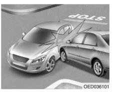
Front air bags may not inflate in side impact collision, because occupants move to the direction of the collision, and thus front air bag deployment does not provide proper protection.
