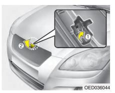
2. Go to the front of the vehicle, raise the hood slightly, push the secondary latch (1) inside of the hood center and lift (2) the hood.
