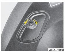
Remove the service cover by turning the plastic screw counterclockwise and removing the cover.
