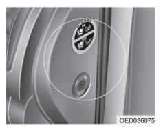
Front passenger's air bag ON/OFF switch (if equipped)
