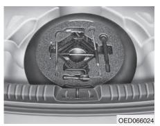
The spare tire, jack, jack handle, wheel lug nut wrench are stored in the luggage compartment. Move the carpeting out of the way to reach this equipment.
