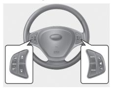
CH ▲/ CH ▼ . . . . Radio mode : Select preset up/down from the preset list of the current waveband
