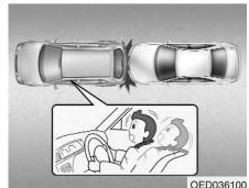
Air bags may not inflate in rear collisions, because occupants are moved backward by the force of the impact. In this case, the air bags do not provide proper protection.
