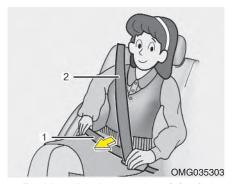
4. Position the lap portion (1) of the belt across your lap as LOW ON THE HIPS as possible to reduce the risk of sliding under it during an accident. Adjust the belt to a SNUG FIT by pulling up on the shoulder portion (2) of the seat belt. The belt retractor is designed to take up excess webbing automatically and to maintain tension on the belt. For your safety do not put any excess slack into the seat belt.
